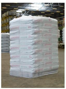
Plasthill stretch hood; prevents transport damage
